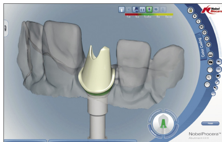
NobelProcera Software for the design of custom abutments includes valuable visual information on the abutment/gingiva interface.
